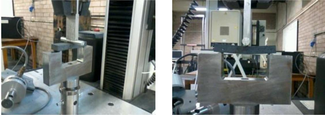
**Figure 4:** Sample mounted for the flexural test in the Instron 5564 device.
