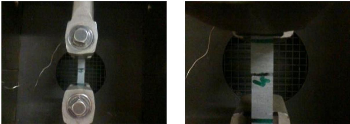
**Figure 1:** Images of the samples gripped in the tensile testing device.
