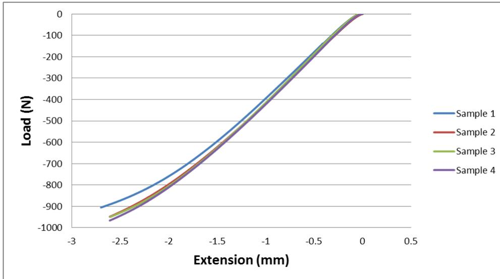
**Figure 5:** Flexural test graph showing the extension of the sample as a function of load.
