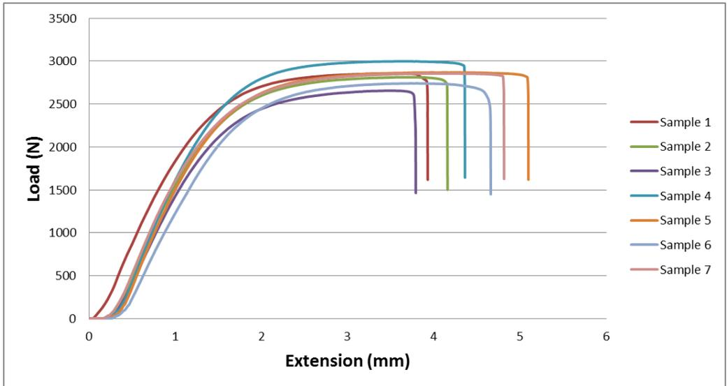
**Figure 2:** Tensile test graph for samples 1 to 7 showing the extension point at brake as a function of load.
