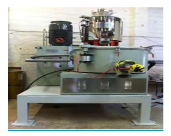
To blend all the ingredients together and also heat the material to remove all moisture and unwanted gases. The surface reaction process occurs at this point (which facilitates material bonding later on in the process). This system also cools the material to the required temperature for further processing
