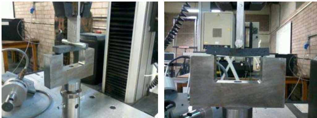
Figure 1: Sample mounted for the flexural test in the Instron 5564 device
